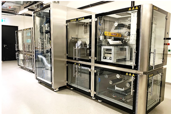
Image 2: Starting in summer 2021, laser processes for battery production will be investigated at Fraunhofer ILT in a dedicated battery center. In the picture: a roll-to-roll plant. © Fraunhofer ILT, Aachen, Germany.
